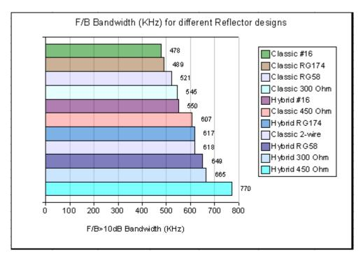
There are no surprises here: the fatter the wire the better the bandwidth, and the Hybrid shape outperforms the Classic shape for each wire type. Some of the arrangements are more practical than others: the 2-wire Classic combination delivers good performance, but its tuning is quite unpredictable; the Hybrid shape using 450 Ohm window does best of all, but construction is more difficult with this type of wire.
