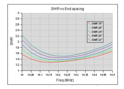
The cardioidal pattern with its narrow "notch" begins to develop with End Spacing values between 24" and 28". So if we opt for a more "modest" spacing, like 24", we shall lose little practical F/B performance and will keep the SWR below 2:1 across the band.
