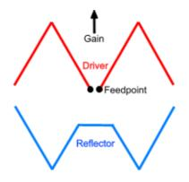
I constructed and evaluated a 10m beam using the Hybrid geometry for the reflector. It showed promise, so I next combined it with the various "fatter" wire options. In all, a total of 11 combinations of wire type and Classic/Hybrid shape were built and tested. The measured F/B>10dB bandwidths are presented below:
