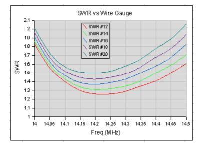
The thicker wire tunes the driven element slightly higher in frequency and with it the minimum SWR; but any "skew" at the band edges - which became a problem when we shortened the driven element - is more than offset by the significantly lower SWR overall.
