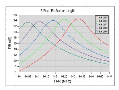
We see that for each 1" increase in Reflector length the frequency of peak F/B drops by about 70KHz, indicating that the beam tuning is linearly dependent on reflector length. A more detailed analysis of the results shows that peak F/B on the reference model occurs at 14.184 MHz, about 100 KHz (0.7%) above the self-resonant frequency of the reflector
