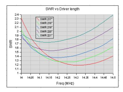
The shortest driven element value (217") produced the lowest SWR; however, bearing in mind that the F/B performance is centred within the band, and that forward gain peaks below the bottom band edge, the shortest value may not be the best choice operationally. The 219" driven element might be a better choice: it produces an SWR curve that is better centred, and its minimum SWR is not unacceptably worse at 1.37:1 vs. 1.19:1.
