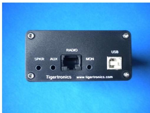
By cutting the PCB track it was simple to disconnect the SPKR port from the AUX port and the input stage of the soundcard, leaving it free to be connected directly to the DATA line via the RJ-45 connector internal wiring. The PCB is conveniently provided with a mini patch panel. So (taking one of the Signalink provided patch links) Pin 5 of the RJ-45 can be connected to the SPKR port.
