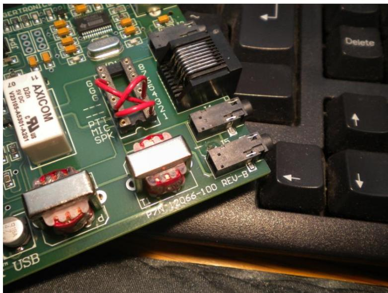
This view also shows the cut in the PCB track (see step 2)
