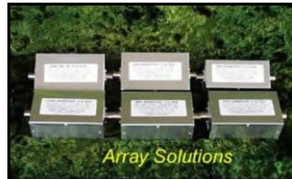
W3NQN Original mono-band band pass filters
